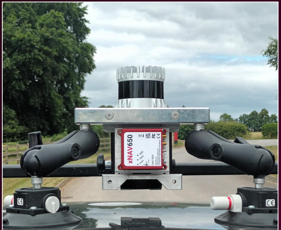
Panpro's LiDAR system includes an OxTS xNAV650 and Ouster LiDAR sensor
